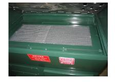
Remove to clean: Lift up and remove the top, to remove the metal mesh filter.
