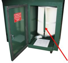
The filter spring holds filter tight to create a seal to prevent "blow by"
