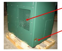
Exhaust air exits the machine in the back
