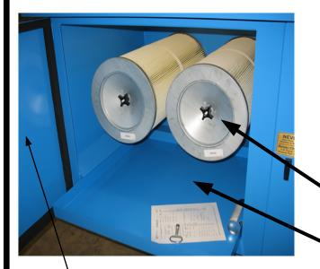
The filters will clean better with the machine off. You may shut the machine off and before it slows down to a complete stop, pulse the filter and allow the fan to prevent the dust from exiting the filter compartment. Filter replacement number is on the gold sticker on the outside of the machine. Be sure to replace with same type of filter or a filter made of polyester media.
