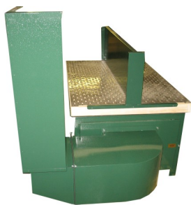
7200B with Dual Workstations and Angled Muffler to keep from impeding workflow
